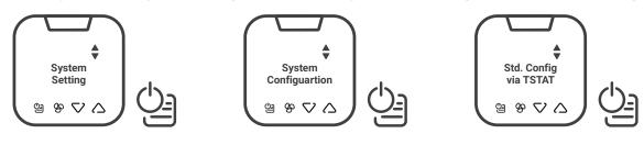
2. Use the Up/Dn arrows to select the type of PTAC you will be controlling. You can choose between "Conventional System" and "Heat Pump System", then tap the Power/Menu key to select.
