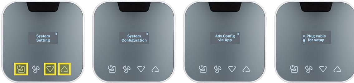
3. Plug the USB-C cable into the thermostat.
