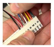
Using wire-nuts, attach the VTech Wiring Harness to the corresponding jumper wires for each pin on the Amana connector, then securely re-attach the wire housing to the control board.
