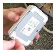
Use the included mounting hardware to mount the thermostat wall plate to the wall, then secure the thermostat to the wall plate using the security screw. The installation is complete.
