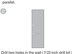
If you drill the holes into a stud, go to step 3. If you drill the holes into an object other than
