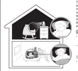
The baby unit has infrared LEDs that allow you to see your baby clearly at night or in a dark room. When the baby unit being viewed detects low light levels, the infrared LEDs are switched on automatically. The images from the baby unit are in black and white, and 2 ppears on the screen.
