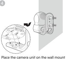
bracket, and then slide it forward until it locks into place. Connect the power adapter to the camera unit and a power supply not controlled by a wall switch.
