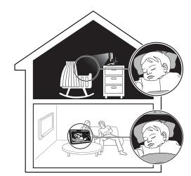
The baby unit has infrared LEDs that allow you to see your baby at night or in a dark room. When the baby unit detects low light levels, the infrared LEDs turn on automatically. The images from this baby unit is in black and white, and J appears on screen.
