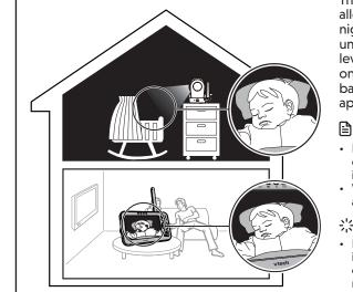
The baby unit has infrared LEDs that allow you to see your baby clearly at night or in a dark room. When the baby unit being viewed detects low light levels, the infrared LEDs are switched on automatically. The images from the baby unit are in black and white, and < appears on the screen.
