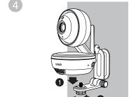
Place the baby unit on the wall mount bracket. Tighten the screw into the threaded socket at the bottom to secure the baby unit.
