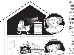
allow you to see your baby clearly at night or in a dark room. When the baby unit being viewed detects low light levels, the infrared LEDs are switched on automatically. The images from the baby unit are in black and white, and <ppears on the screen.
