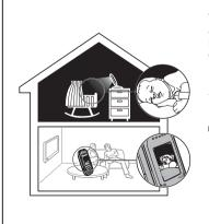
The baby unit has infrared LEDs that allow you to see your baby at night or in a dark room. When the baby unit detects low light levels, the infrared LEDs turn on automatically.
