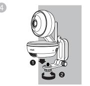
Place the baby unit on the wall mount bracket. Tighten the screw into the
