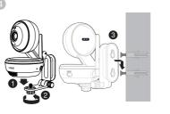
Place the baby unit on the wall mount bracket. Tighten the screw into the threaded socket at the bottom to secure the baby unit. Align the holes on the wall mount bracket with the screws on the wall, and slide the wall mount bracket down until it
