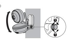
The default angle of the wall mount bracket is 90 degrees. You can maximize your baby unit's viewing angles by tilting the wall mount bracket.
