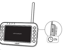
Press any keys on the parent unit to turn on the screen again
