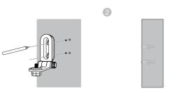
Check for reception strength and camera angle before drilling the holes.
