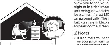
The baby unit has infrared LEDs that allow you to see your baby clearly at night or in a dark room. When the baby unit being viewed detects low light levels, the infrared LEDs are switched on automatically. The images from the baby unit are in black and white, and
