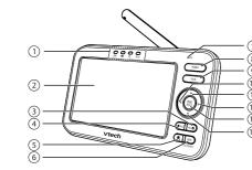
LED lights Indicate the different statuses of the parent unit. For details, refer to **Parent**
