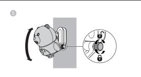
The default angle of the wall mount bracket is 90 degrees. You can maximize your baby unit's viewing angles by tilting the wall mount bracket.
