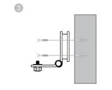
Align the wall mount bracket and screws with the holes in the wall as shown. Tighten the screw in the middle hole first, so that the wall mount bracket position is fixed. You can tighten the other screw in the top hole.
