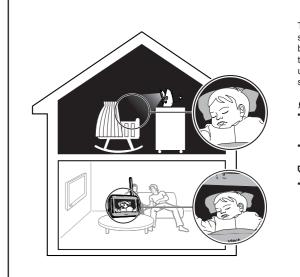
The baby unit has infrared LEDs that allow you to see your baby at night or in a dark room. When the baby unit detects low light levels, the infrared LEDs turn on automatically. The images from the baby unit are in black and white, and J appears on
