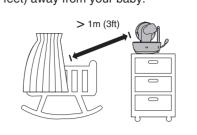
Place the parent unit more than 1 meter (3 feet) away from the baby units.
