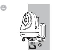
Place the baby unit on the wall mount bracket. Tighten the screw into the threaded socket at the bottom to secure the baby unit.
