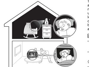
The baby unit has infrared LEDs that allow you to see your baby clearly at night or in a dark room. When the baby unit being viewed detects low light levels, the infrared LEDs are switched on automatically. The images from the baby unit are in black and white, and appears on the screen.
