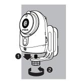
Place the baby unit on the wall mount bracket. Tighten the screw into the threaded socket at the bottom to secure the baby unit.
