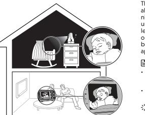
The baby unit has infrared LEDs that allow you to see your baby clearly at night or in a dark room. When the baby unit being viewed detects low light levels, the infrared LEDs are switched on automatically. The images from the baby unit are in black and white, and appears on the screen.
