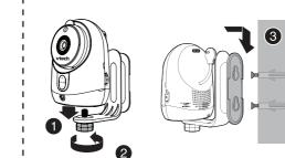
Place the baby unit on the wall mount bracket. Tighten the screw into the threaded socket at the bottom to secure the baby unit. Align the holes on the wall mount bracket with the screws on the wall, and slide the wall mount bracket down until it locks into place.
