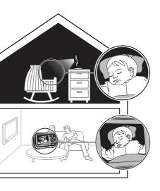
The baby unit has infrared LEDs that allow you to see your baby clearly at night or in a dark room. When the baby unit being viewed detects low light levels, the infrared LEDs are switched on automatically. The images from the baby unit are in black and white, and 🕥 appears on the screen.
