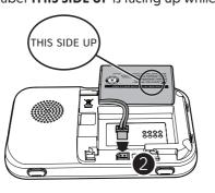
3. Push the battery compartment cover back until it secures into place.
