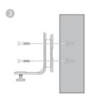
Align the wall mount and screws with the holes in the wall as shown. Tighten the screw in the middle hole first, so that the wall mount position is fixed. You can tighten the other screw in the top hole.
