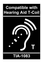
Telephones identified with this logo have reduced noise and interference when used with most T-coil equipped hearing aids and cochlear implants. The TIA-1083 Compliant Logo is a trademark of the Telecommunications Industry Association. Used under license.
