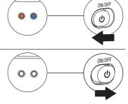
🖹 Note • Slide the  $\bigcirc$  ON/OFF switch rightward to power off your HD camera.
