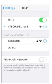
4. Tap to select your preferred and secured 2.4GHz Wi-Fi network for your IP camera. You must select the same Wi-Fi network that your mobile device has connected to.
