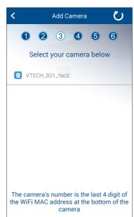
5. Tap to select your preferred and secured 2.4GHz Wi-Fi network for your IP camera. You must select the same Wi-Fi network that your mobile device has connected to.
