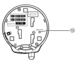
13 – Pair/reset button Press and hold for three seconds to enter pairing mode
