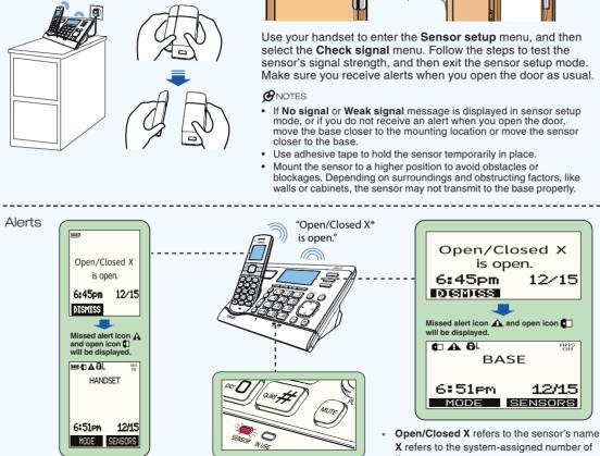
Test the sensor signal strength
