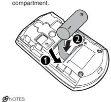
• Use only CR123A lithium battery. • While you insert the battery, make sure the polarities are correct.
