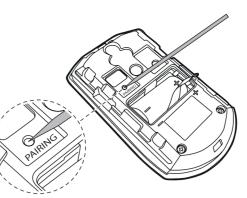
When the registration process completes, the green LED light on the sensor will remain steady for about two seconds, and then turn off. The registration process takes about 90 seconds to complete.
