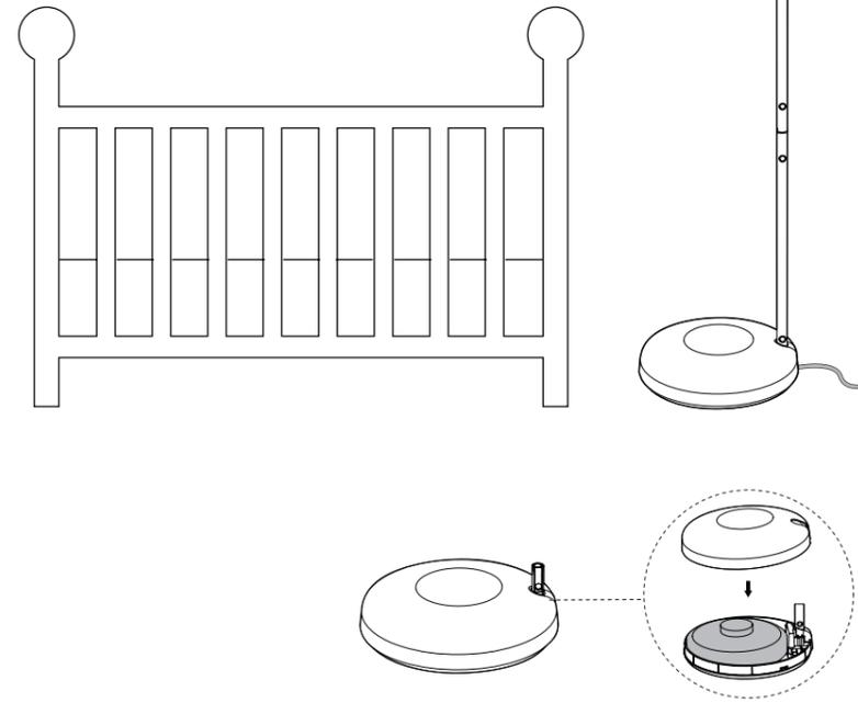
8. Install the Baby Unit onto the First extension (A). Connect the adapter to the end of the cable and the power supply to power up the Baby Unit. Slide the switch to **ON** to power your Baby Unit on.
