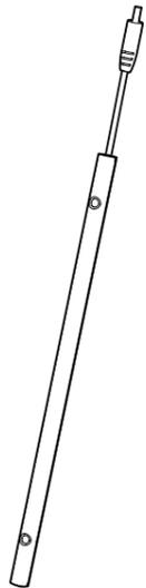
4. Pass the cable jack through the connector pipe (B), the second pole, the second connector pipe (B), and the third pole in turn. Align the slot between the poles and connector pipes (B) and connect all three poles firmly with the pipes.
