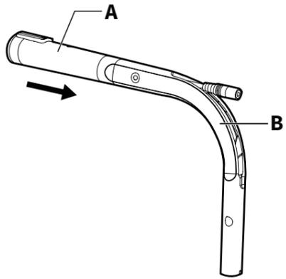
2. Let the cable jack of the Extension cable pass through from the back of the base.
