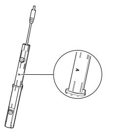
Pass the cable jack through the Second extension (B), to the opening.
