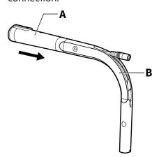
3. Pick one pole and pass the cable jack through the pole, then connect the pole with the Base.
