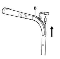
6. Connect the cable jack with the DC socket, then secure the cable with the Extension cover (C).
