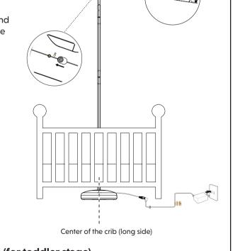
Installation with table stand (for toddler stage) Connect the baby unit power connector to the table stand, then plug the power adapter to the power jack and a power supply.
