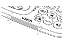
2. <u>Press and hold</u> the pair button **W** on the right side of the Extension ringer until the 🗲 green LED light on the front flashes, then release 🏜.
