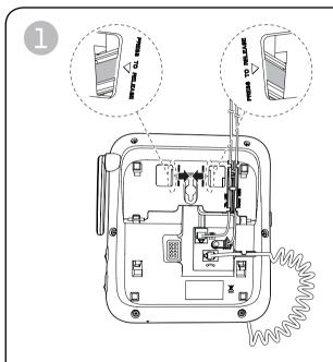
Press the tabs of the wall-mount bracket to release it from the tabletop orientation.
