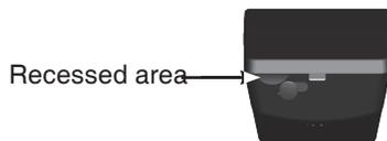
3. Use your thumb to slide along the sides of the handset carefully to release the tabs on the handset cover from the slots on the sides of the handset. Then gently detach the handset cover from the handset.
