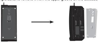
3. Turn the mounting bracket upside down. Insert the small tabs on the mounting bracket into the upper slots on the accessory Petite. Then press the large tab on the mounting bracket and firmly push it into the lower groove on the accessory Petite.
