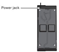
2. Position the mounting bracket as shown. Insert the two small tabs of the mounting bracket into the lower slots on the accessory Petite. Then press the large tab on the mounting bracket and firmly push it into the upper groove on the accessory Petite.
