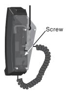
3. Plug the Cat-5 network cable into the network wall jack with Power over Ethernet (PoE). Then connect the coiled handset cord to the telephone base.
