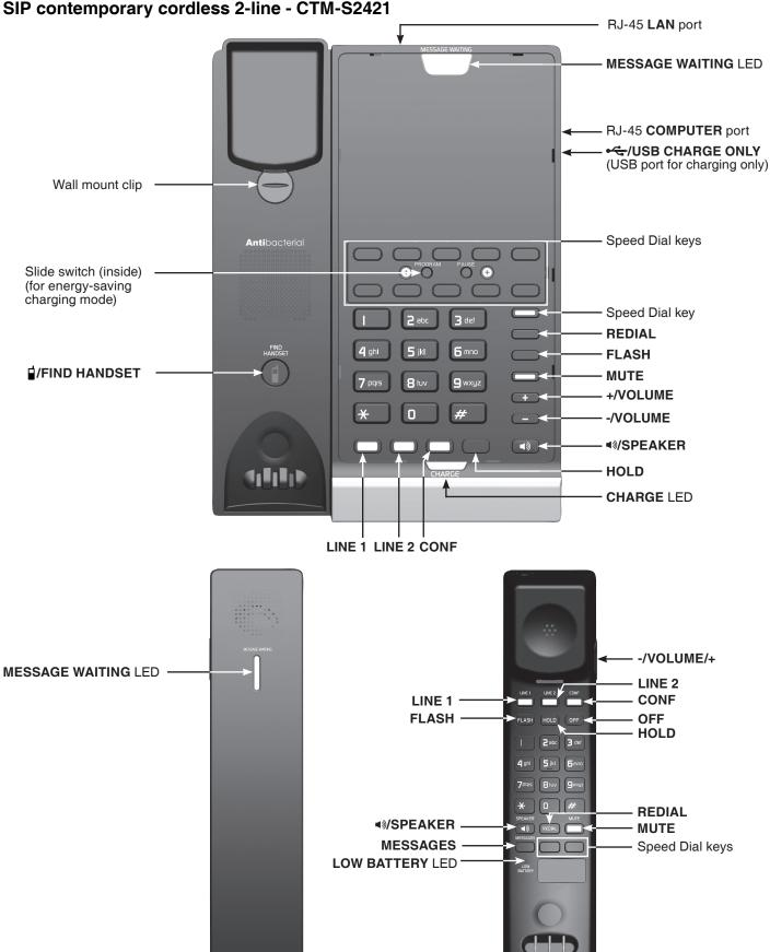
NOTE: Keep the slide switch (inside the phone) on the left side to maintain normal telephone operation.
