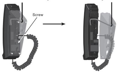
4. Rotate the mounting bracket. Insert the tabs of the mounting bracket into the lower grooves of telephone base. Then tighten the screw to affix the mounting bracket.
