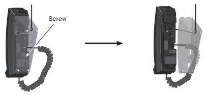
4. Rotate the mounting bracket. Insert the tabs of the mounting bracket into the lower grooves of telephone base. Then tighten the screw to affix the mounting bracket.
