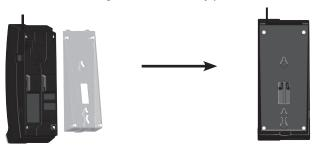
4. Mount the accessory Petite on the wall by aligning the eyelets with the mounting studs of the wall plate. Then slide the accessory Petite down on both mounting studs until it locks into place. Place the handset on the accessory Petite cradle.
