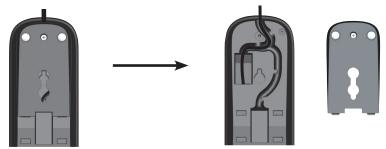
4. Rotate the mounting bracket. Insert the tabs of the mounting bracket into the lower grooves of the telephone base. Then tighten the screw to affix the mounting bracket.
