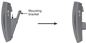
4. Mount the telephone base on the wall by aligning the eyelets with the mounting studs of the wall plate. Then slide the telephone base down on both mounting studs until it locks into place.
