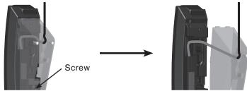
4. Rotate the mounting bracket. Insert the tabs of the mounting bracket into the lower grooves of the charging base. Then tighten the screw to affix the mounting bracket.
