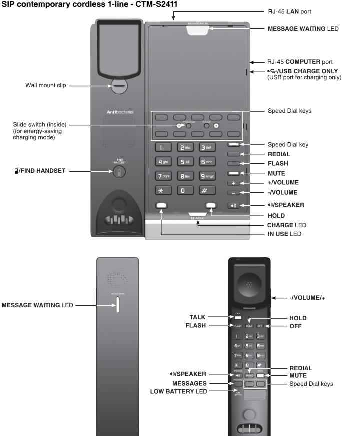
NOTE: Keep the slide switch (inside the phone) on the left side to maintain normal telephone operation.
