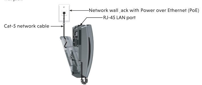
Once installed, the telephone begins a four-step initialization and system registration process.
