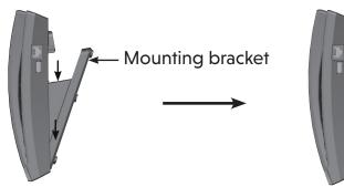
4. Plug the Cat-5 network cable back into the network wall jack with Power over Ethernet (PoE). Then slide the telephone base down on both mounting studs until it locks into place.
