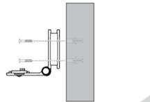
4. Place the camera unit on the wall mount bracket, and then slide it forward until it locks into place. Connect the power adapter to the camera unit and a power supply not controlled by a wall switch.
