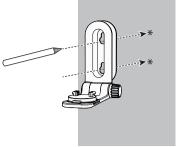
3. Align the wall mount bracket and screws with the holes in the wall as shown. Tighten the screw in the middle hole first, so that the wall mount bracket position is fixed. You can tighten the other screw in the top hole.
