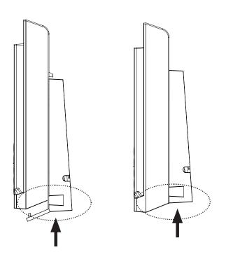
Connect the telephone as described in "Telephone base installation" on page 8, but connect the short Ethernet cable instead. Place the cords in the associated cable ducts. 4. Mount the telephone base on the wall by positioning the eyelets on the telephone base and the mounting bracket against the mounting studs. Then slide the telephone base down on both mounting studs until it locks into place.
