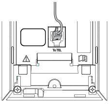
2. Align the grooves of the base stand with the telephone base. Slide the base stand up to secure it.
