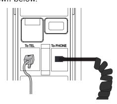
Align the grooves of the base stand with the telephone base. Slide the base stand up to secure it.
