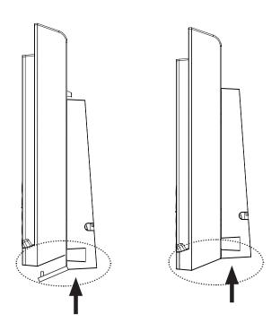
3. Connect the telephone as described in "Telephone base installation" on page 8, but connect the short telephone line cord instead. Place the cords in the associated cable ducts.
