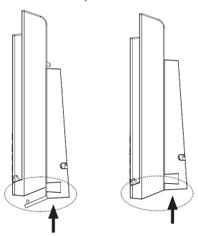
Connect the telephone as described in "Telephone base installation" on page 10, but connect the short telephone line cord instead. Place the cords in the associated cable ducts. 4. Mount the telephone base on the wall by positioning the eyelets on the telephone base and the mounting bracket against the mounting studs. Then slide the telephone base down on both mounting studs until it locks into place.
