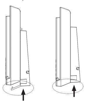
3. Connect the telephone as described in "Telephone base installation" on page 8, but connect the short telephone line cord instead. Place the cords in the associated cable ducts.
