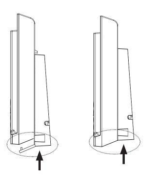
3. Connect the telephone as described in "Telephone base installation" on page 10, but connect the short telephone line cord instead. Place the cords in the associated cable ducts.
