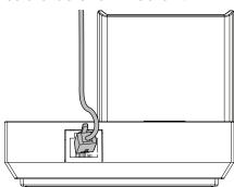
2. Plug the other end of the telephone line cord to the telephone wall jack and the power cord connector to the power adapter. Plug the power adapter to a wall power outlet.
