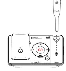
2. The magnet holds the top of the headset in place. The **b** light turns on when charging.
