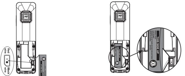
3. Slide the battery compartment cover towards the center of the handset until it clicks into place.
