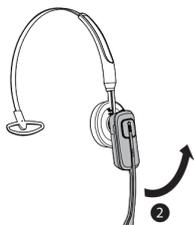
4. Adjust the head band to fit your head. Adjust and rotate the angle of the headset until the microphone is pointing towards your mouth.
