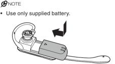
Install the handset battery as shown below.
