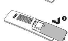
Install the headset battery as shown below.
