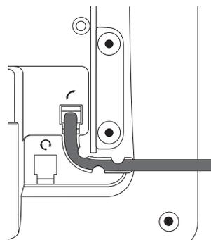
1. Place the top of the grooves on the footstand (Fig. 1) below the slideguides on the back of the phone (Fig. 2). For the upright position, the short "legs" of the footstand must be attached to the phone; for the more horizontal position, use the long ones.
