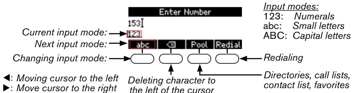
Press any key on the alphanumeric keypad or pick up handset to open the "Enter Number" screen. The current input mode is indicated in the information line underneath the cursor line. Press the left function key underneath the display to switch to the input mode indicated by the symbol directly above it in the function key line.
